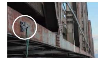
アクセス困難な部位での点検・非破壊評価・振動計測を目的とした検討の例 (ロボティクス) Example of inspections, non-destructive evaluations, and vibration measurements for sections difficult to access (Robotics)
